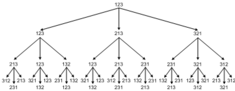
Figure 2 contains the algorithm we used to shuffle our deck of three cards, and also depicts the tree of all possible decks using this shuffling algorithm. If our random number source is a good one, then each leaf on the tree in Figure 2 has an equal probability of being produced.
